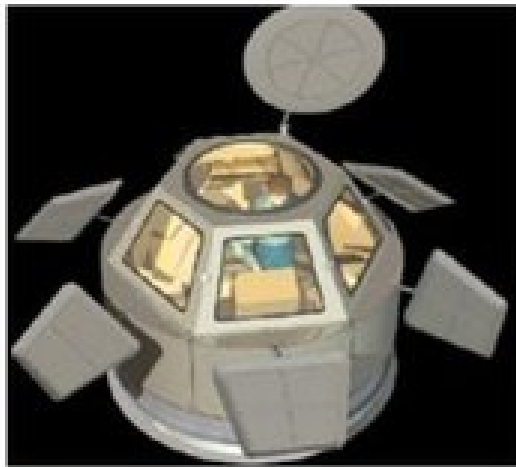
Deployed shutters for Cupola windows.
