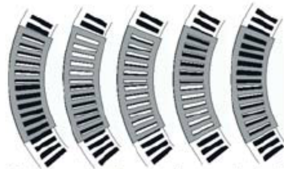
Disc shown against mask, rotated slightly between each picture. Light intensity changes for each detector can be seen.
